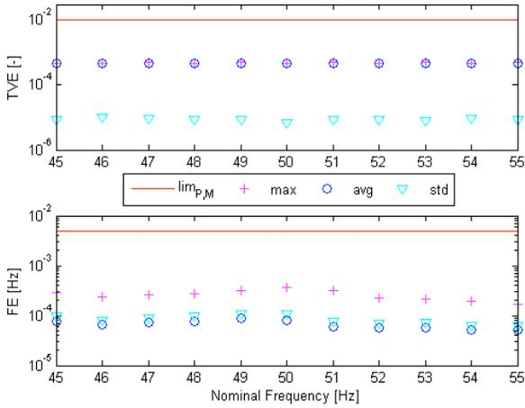
Fig. 2. PMU TVE and FE with reference to static tests with single tone signals.
