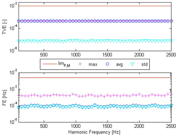
Fig. 3. PMU TVE and FE with reference to static tests with distorted signals.
