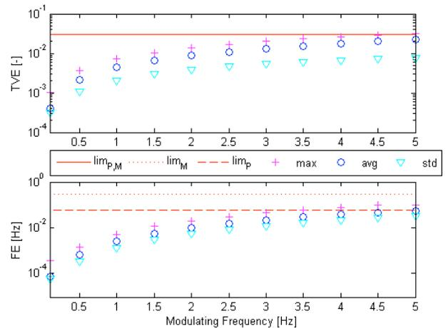
Fig. 5. PMU TVE and FE with reference to amplitude and phase modulations.
