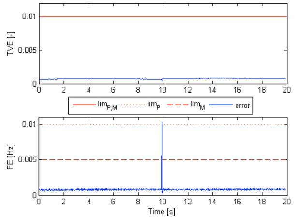
Fig. 4. PMU TVE and FE with reference to the frequency sweep dynamic test.
