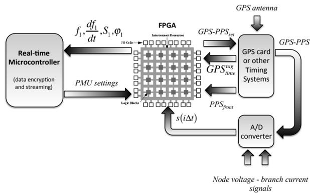
Fig. 1. Implementation of the synchrophasor estimation algorithm into the NI CompactRio embedded system.
